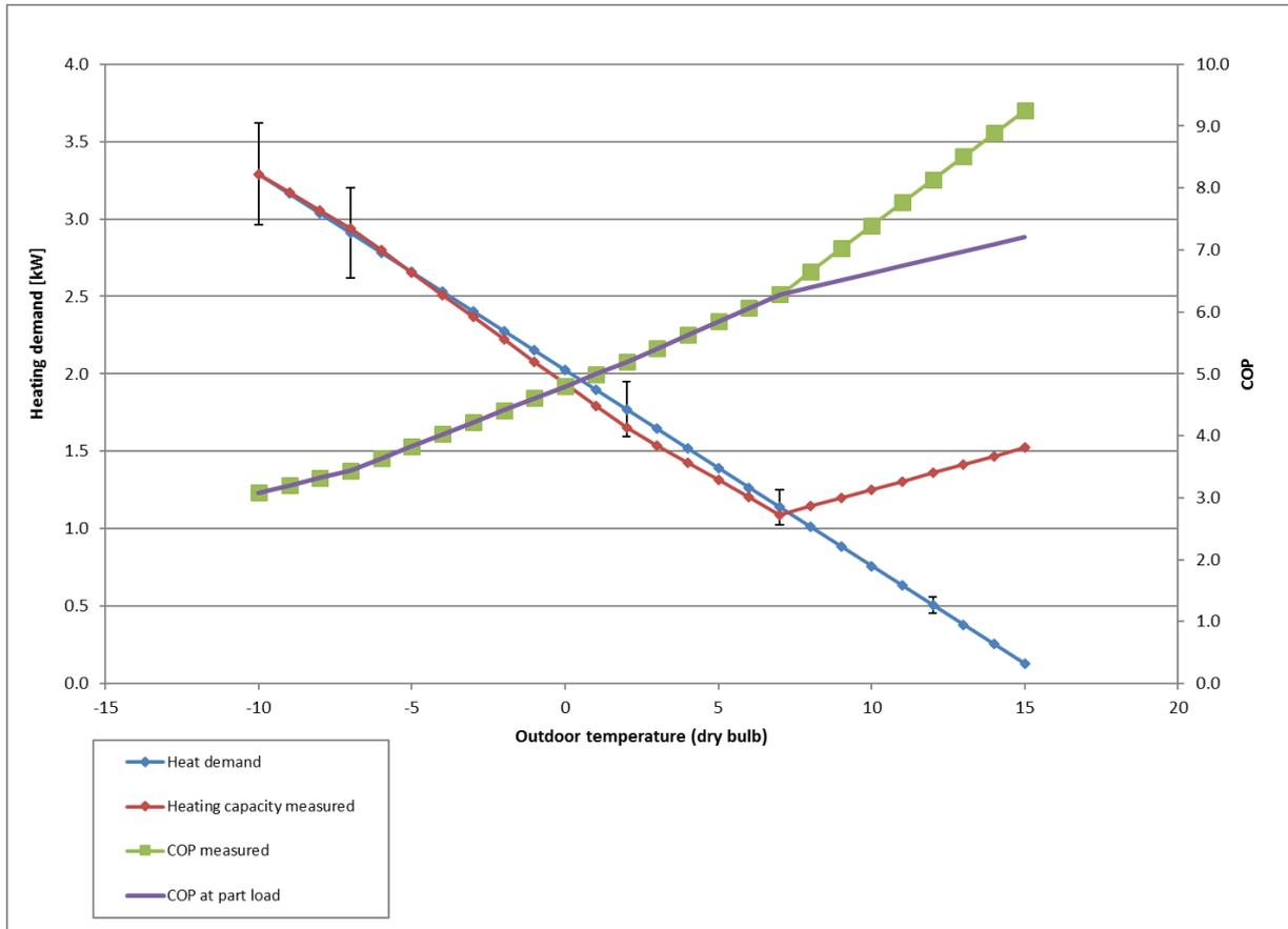
The heating capacity of the heat pump was adjusted by means of the inverter in order to fit within 10 % of the reference heat demand. For part load conditions above 10 % of the heating demand, a degradation factor is applied to the measured COP. For part load conditions below 10 % of the heating demand, electrical heating is applied to reach the full heating demand. The corrected COP is illustrated in the diagram as 'COP at part load'.
